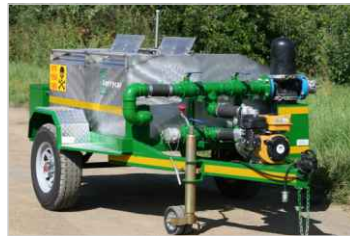
1100L Chemical mixing trailer *Available in 2" or 3" pipe system
