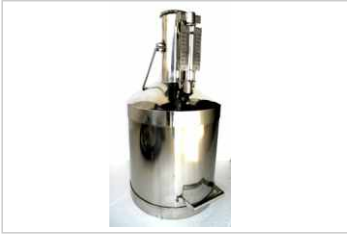
Stainless steel calibrating can (prover) 20L
