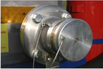
Bottom fill dry break couplers for diesel/petrol and aviation fuels
