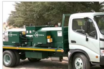
**Custom-made tanks and transfer equipment for diesel and aviation fuels**
