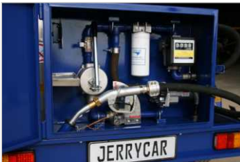
GPI 50L/min pump station with backup GPI piston hand pump • 12 volt (available in 24 volt)
